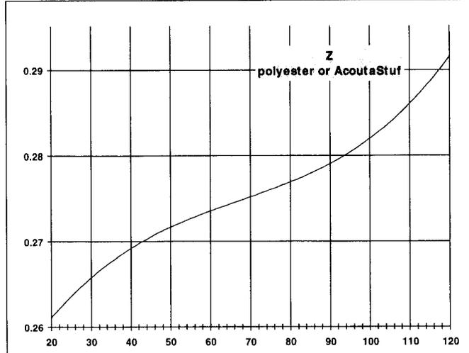
**FIGURE 5:**  $\alpha$ -transmission line Z value—polyester, cotton, AcoustaStuf. The Z value is needed to determine the cross-section area. Using the same pipe frequency, read the Z value from the curve. Use Z in this equation to set proper cross-section:  $S_x$  equals  $Z \times f_s \times f_{\Theta} \times V_{AS} / (10,000 \times \alpha)$ , where  $\alpha$  equals  $\sqrt{1 + (f_{\Theta} / f_s \times Q_{TS})}$ . The shape of the cross-section is up to you.
