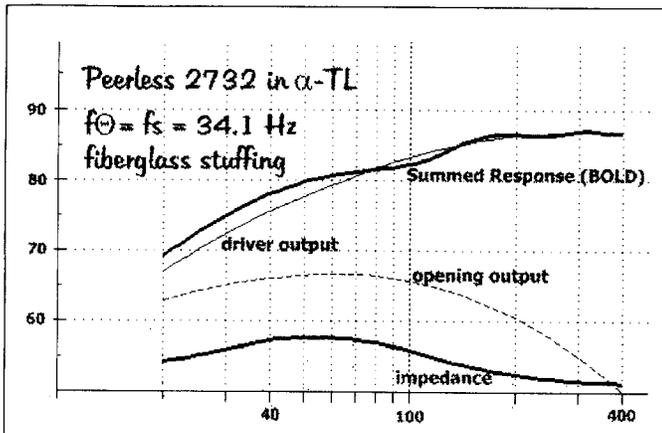
FIGURE 8: Traditional  $\alpha$ -TL using the Peerless 2732. This graph is another example of how quiet long pipes are. The pipe frequency is the same as driver resonance, which is 34Hz. Summed response quiets noticeably below 125Hz. The shelving of response between 50 and 110 is largely due to the  $3\Theta$  resonance. When  $3\Theta$  resonance is better controlled, the shelf would be smoothed out. (Thanks to Peerless, who provided these drivers for an earlier, failed project.)
