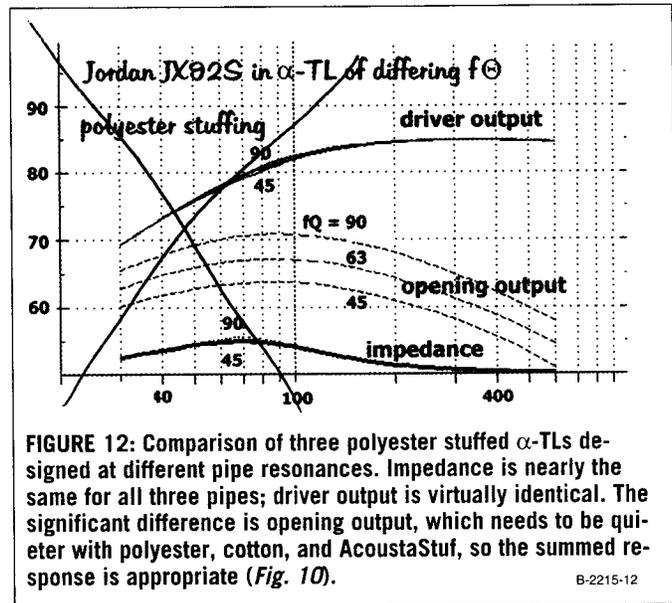
FIGURE 12: Comparison of three polyester stuffed  $\alpha$ -TLs designed at different pipe resonances. Impedance is nearly the same for all three pipes; driver output is virtually identical. The significant difference is opening output, which needs to be quieter with polyester, cotton, and AcoustaStuf, so the summed response is appropriate (Fig. 10).
