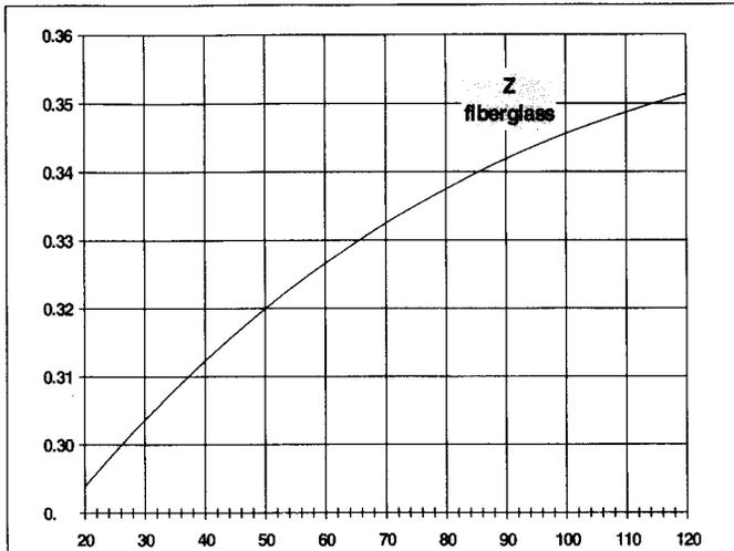
**FIGURE 4:**  $\alpha$ -transmission line Z value—fiberglass. The Z value is needed to determine the cross-section area. Using the same pipe frequency, read the Z value from the curve. Use Z in this equation to set proper cross-section:  $S_x$  equals  $Z \times f_s \times f_{\Theta} \times V_{AS} / (10,000 \times \alpha)$ , where  $\alpha$  equals  $\sqrt{1 + (f_{\Theta} / f_s \times Q_{TS})}$ . The shape of the cross-section is up to you.
